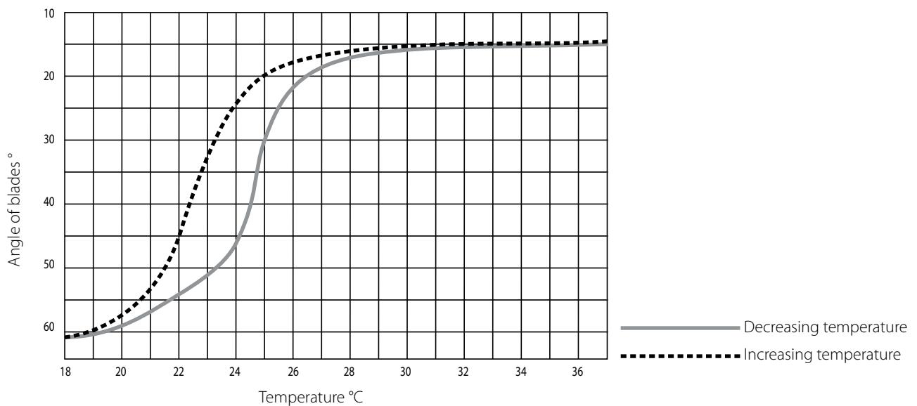
Thermal actuator feels temperature and adjusts angle of the blades automatically. Temperature range is from 18 °C to 36 °C. Additional source of energy and electric installation is unnecessary.
