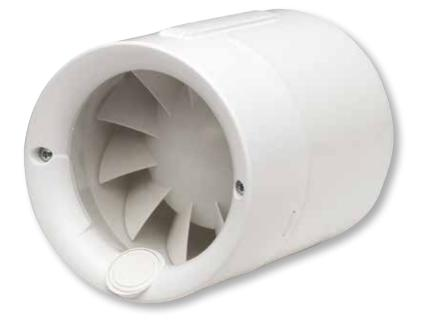
Transfer axial fan offering a very low noise level and specifically designed to work through a duct or to be flush mounted into the wall, ideal for ventilating small areas or to exchange heat between adjoining rooms. Fitted with single phase motors 230V-50Hz, IP44, Class II, with ball bearings for enhanced working life and assembled on silent-blocks.
