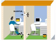
SILENTUB-100 can be flush mounted into the wall, ideal for ventilating small areas or to exchange heat between adjoining rooms.
