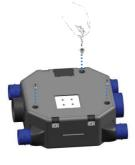
Remove the 3 screws TORX T40 (with hexagonal head 10 mm) in the cover
